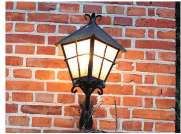
Figure E.12: NonFCO, frosted glass. UH: 15-20%, UL: 5-10%, ULR: 20-30%
